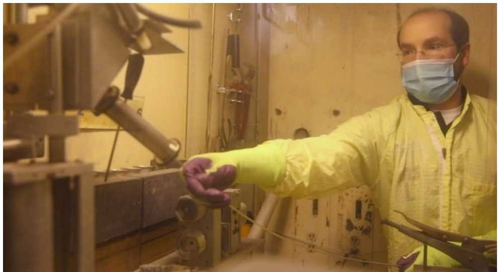
Figure 2 – Rabbit containing ^{176}\text{Yb} being inserted into MIT Nuclear Reactor
